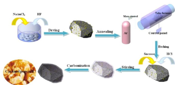
Figure 1. Schematic depiction of the fabrication process for caramel popcorn shaped Si-C particles.
